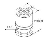
Fixing plate: zinc alloy, chrome-plated Tube: stainless steel, black powder coated
